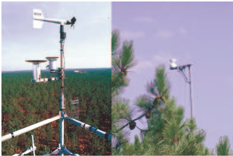
figure II.2.3-a : left: mean wind speed and direction, air temperature and humidity; right: rainfall measurements over a maritime pine forest measurement site (Le Bray site).
