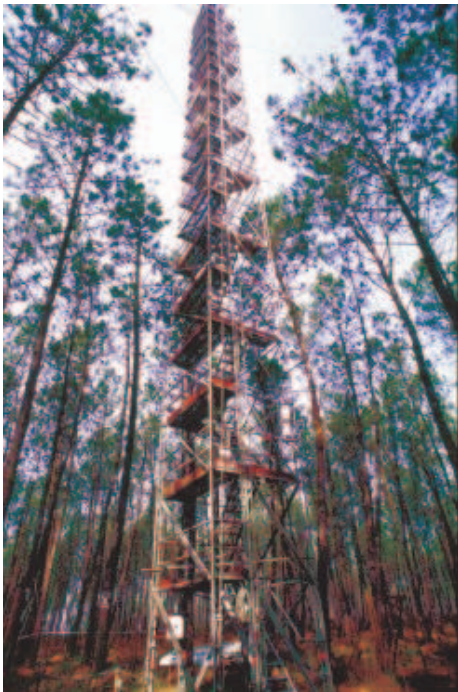
figure VI.5.1-a : Le Bray site equipped with a 40 m high scaffolding with EC and meteorological measurements
