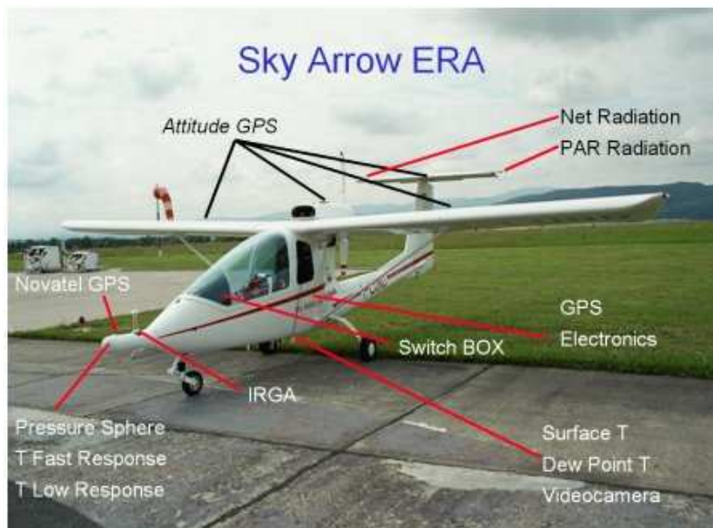
figure VI.1.2-a : Photograph of the SkyArrow ERA showing the exact location of the sensors and instruments mounted onboard.
