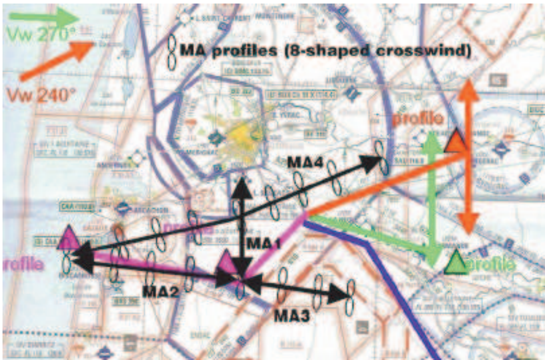
figure III.2.5.2-a : MetAir's basic flight legs MA1 through MA5 shown together with the existing design of the pattern "Landes" for the Aztec
