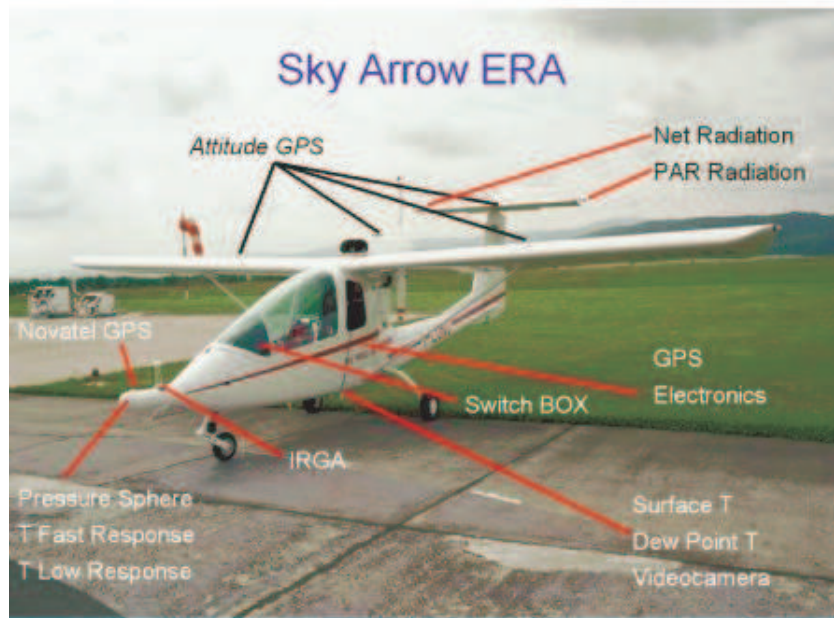
figure III.2.3-a : Photograph of the SkyArrow ERA showing the exact location of the sensors and instruments mounted onboard.
