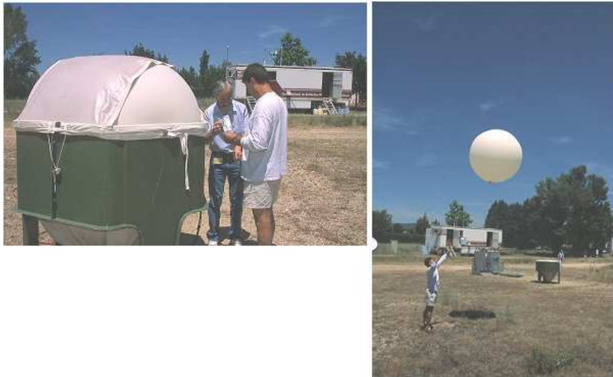
figure III.1-a : Preparation and release of a radiosonde balloon
