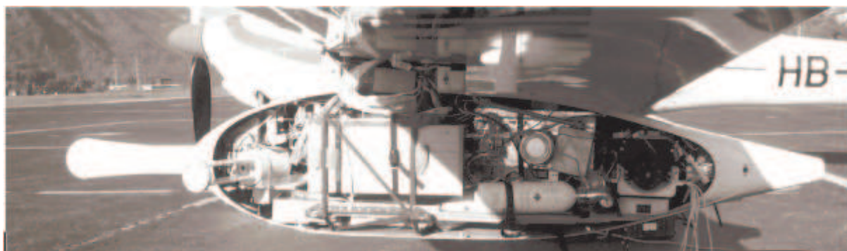
figure VI.1.4-b : One of the two pods densely packed with instrumentation
