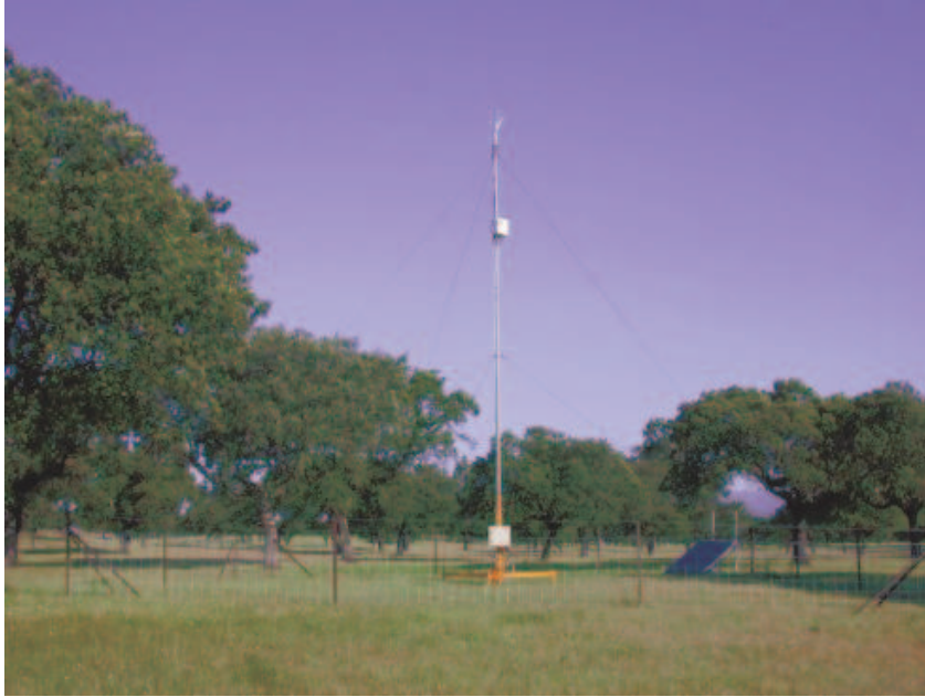
figure VI.5.5-a : Eddy Correlation System
