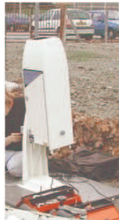
figure II.3.2-a : Vaisala CT25K ceilometer
