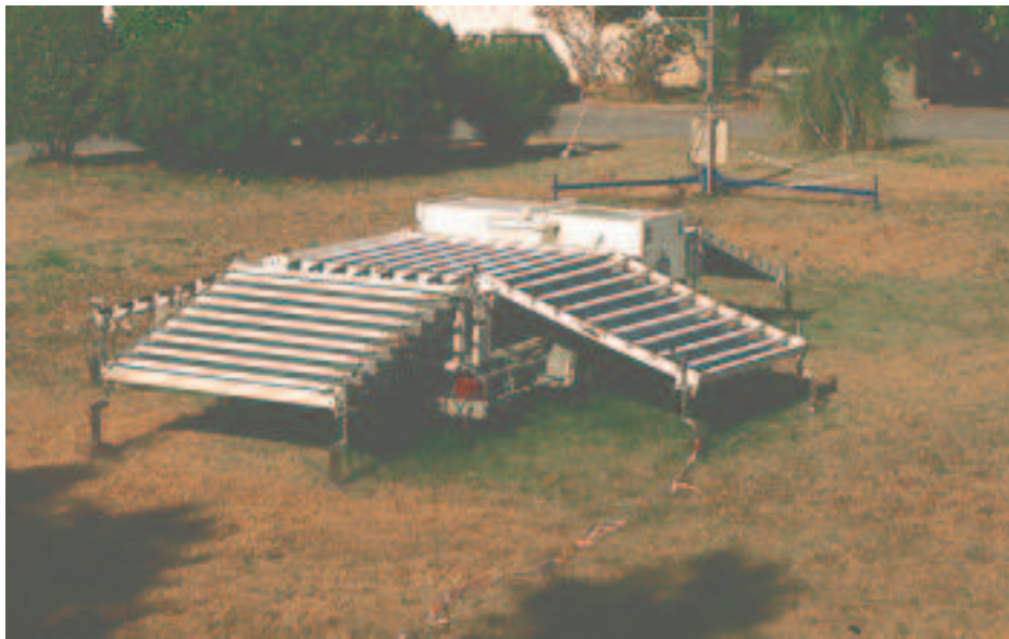
figure II.3.1-a : The UHF Degreane PCL1300 wind profiler
